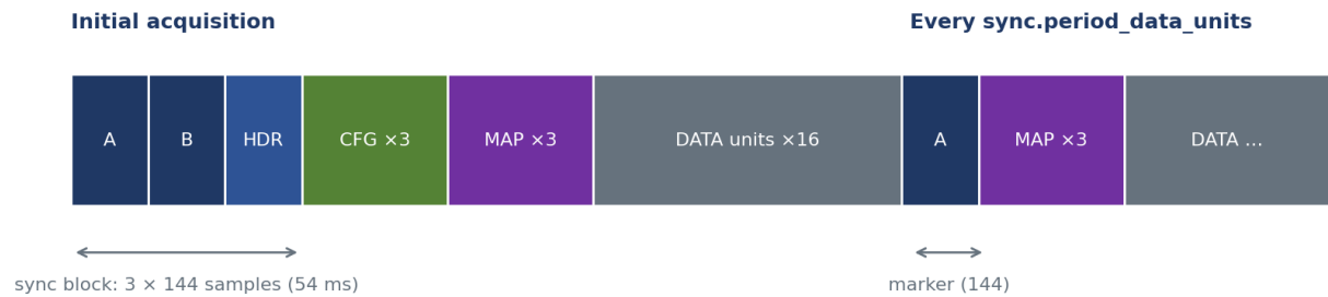
Figure 1. On-air framing: initial acquisition (sync block + config/map descriptors) and the recurring mid-stream marker context.
